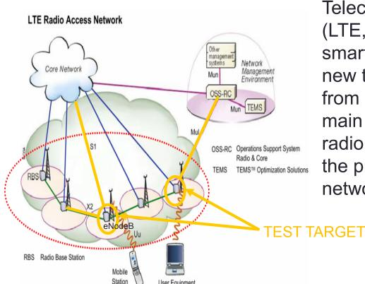
Telecommunications network (LTE, 4G) with all-IP network and smart terminals will introduce new threat scenarios triggered from radio network side. The main test target initially were radio base stations but during the project different types of network nodes were tested.
